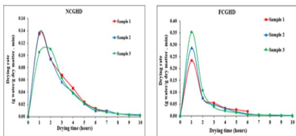
Figure 2. Variation of drying rate with respect to drying time for the drying of groundnut samples under NCGHD and FCGHD modes
