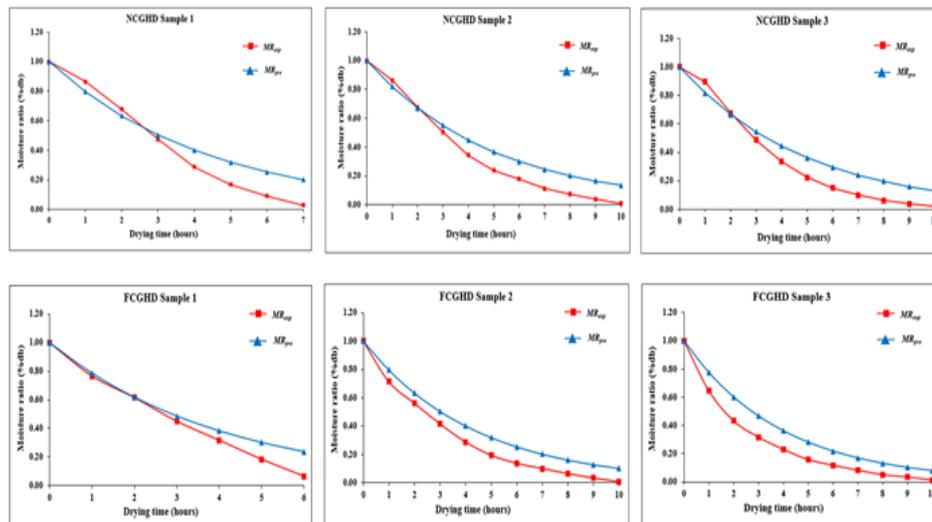
Figure 1. Variation of moisture ratio with respect to drying time for the drying of groundnut samples under NCGHD and FCGHD modes
